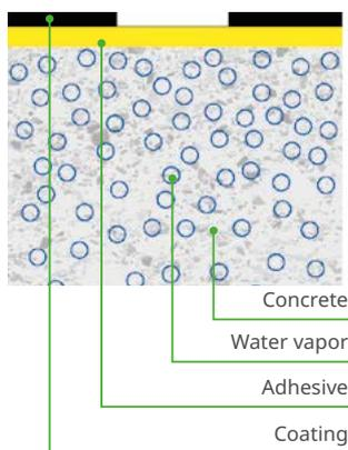
When a floor coating is applied, it typically has a higher diffusion resistance than concrete.
