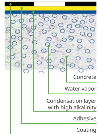
Once such a highly alkaline condensation layer has formed under a vapor-tight, firmly bonded coating, the primer and adhesive are directly exposed to this aggressive environment. Due to the moisture and the high pH value, the adhesive can degrade over time.
